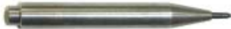
Stylus holder for sharpening. This allows you to use a grinding wheel without burning your fingers.
